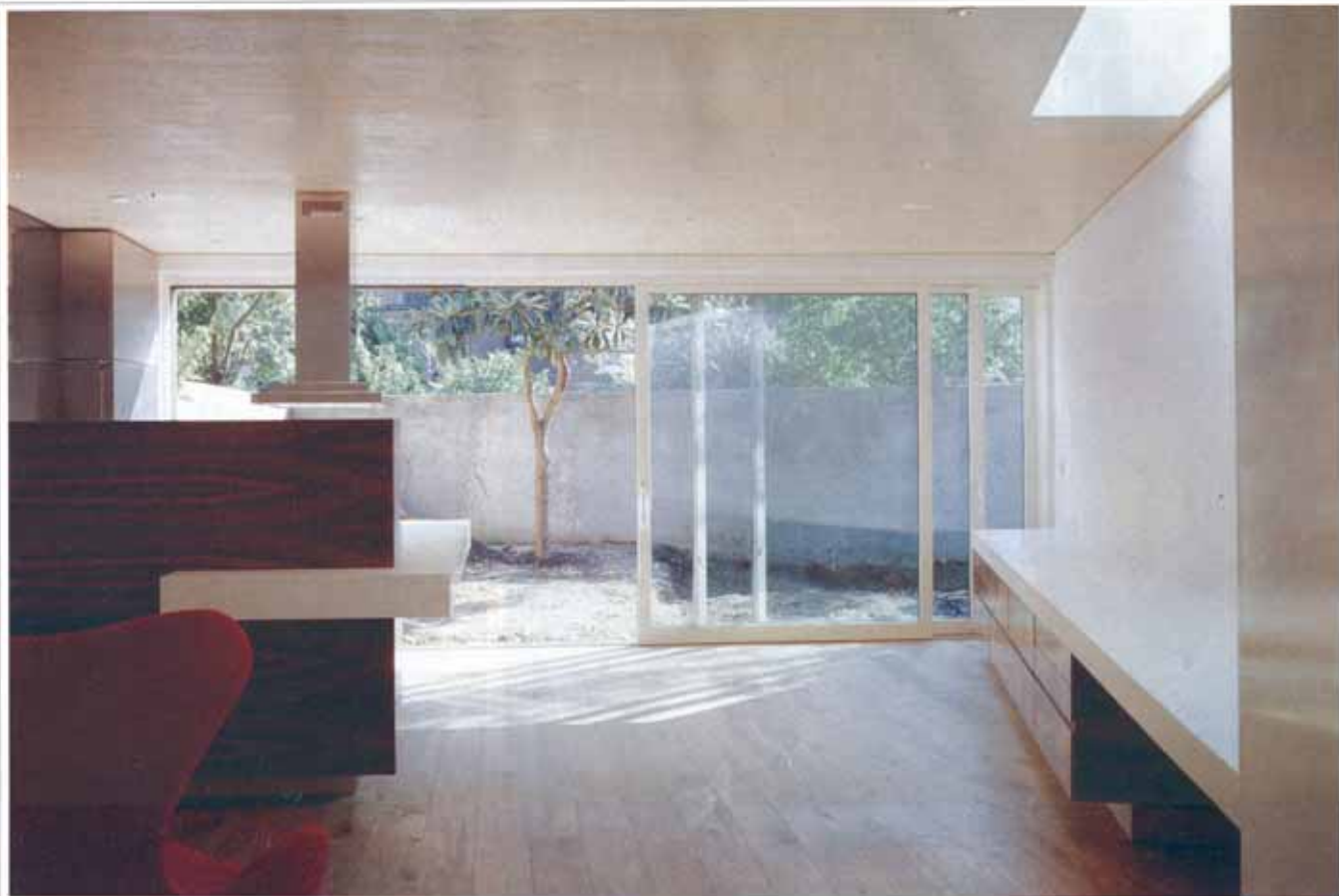
Left: Looking out from the ground floor kitchen/living space. The large window areas will ideally be protected by external louvers in the summer and by internal curtains in the winter. Below left: Staircase.
