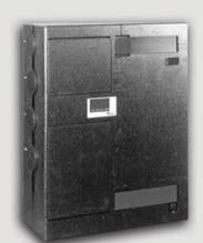
This unit saves heat from the internal air produced by solar gains, people and electric items to pre-heat a supply of fresh air. If air heating is not required only fresh filtered air is supplied. These filters need to be replaced every 6months in london. The system saves about 10 times more energy than it uses! It is located in the store in an insulated cupboard.
